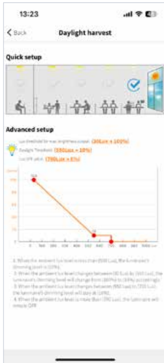
Figure 6.8 Daylight harvest setup
